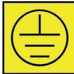
Grounding label: serves as marker to attach a grounding disk while assembling the system
